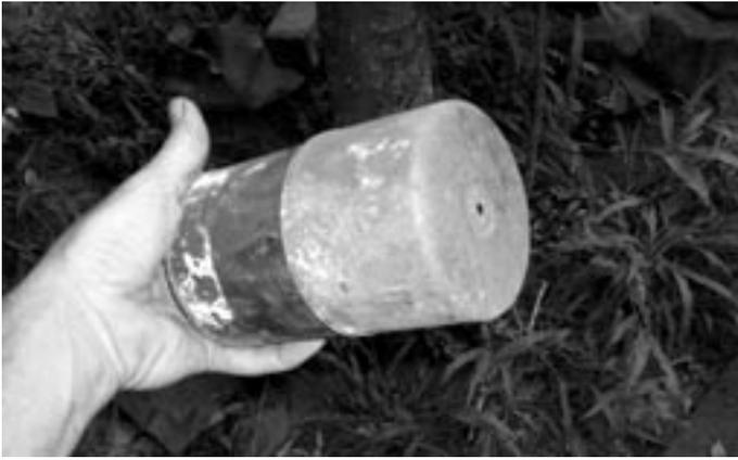
Pic 1. Up to 300g: Small tins in a woodstove. These are two tins that fit tightly over each other, after one end is taken out of each tin. A hole is punched in one tin with a 3" nail.
