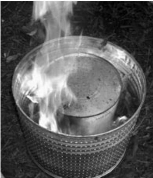
Pic 5. 3-6 kg: Stainless Fisher & Paykel drum provides lots of secondary air with all those holes, and is a good size for a 20 litre paint tin retort. This unit makes a great carbon-negative space heater, and more than a 'one-person-day' CO<sub>2</sub> footprint's worth of charcoal for sequestration.
