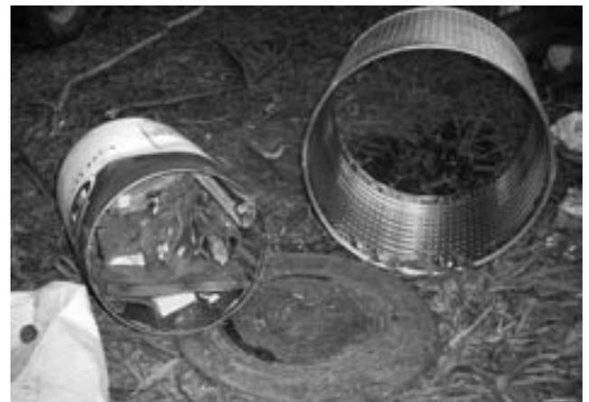
Pic 6. Components for the Guenther inverted-drum technique, including base plate and 20-litre drum charged with wood. Smaller fuel size is better, less than 50mm is best.
