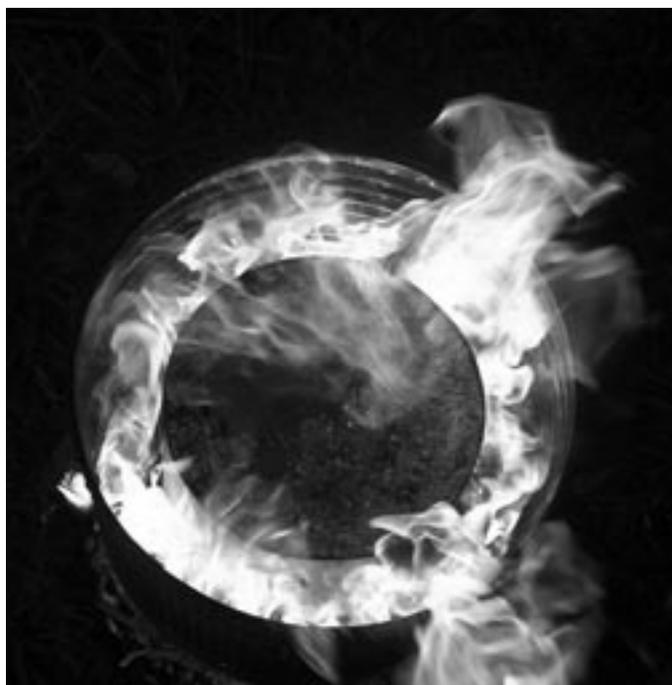
Pic 8. The woodgas lights up and burns vigorously for 30 minutes or more. The primary fire is kept going for another 30 minutes, after the last woodgas flames are visible, to ensure all the gases are driven off. Yield is >40% of EMC weight. This is the basic unit to replicate for a Jagama-style climbing kiln. Insulation and walls raise efficiency, and are up to you.
